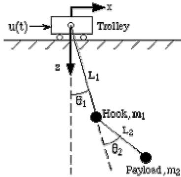
Fig. 5. Double pendulum model of a crane system
