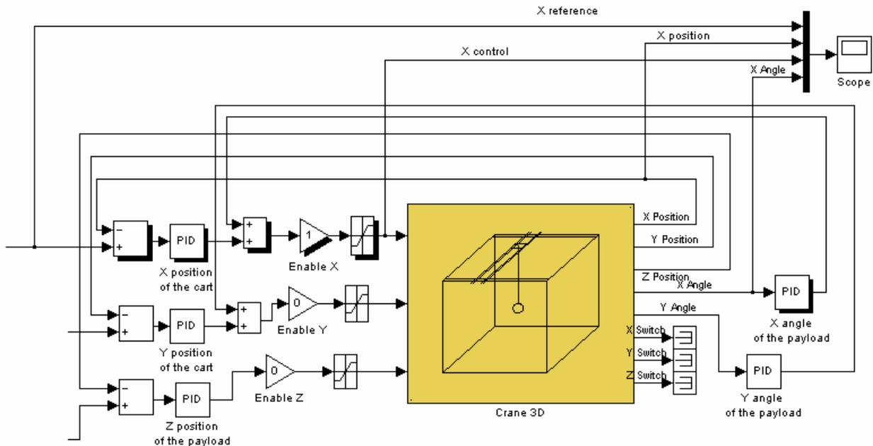
Fig. 18. Matlab control of crane load [5]
