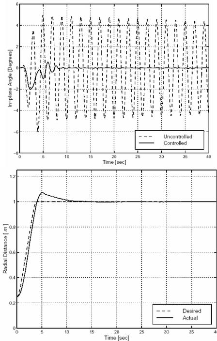
Fig. 9. Crane load angle and distance response
