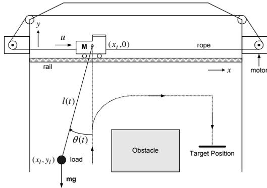
Fig. 19. A schematic diagram of container crane systems for obstacle avoidance
