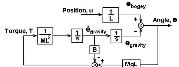
Fig. 12. Crane trolley control scheme
