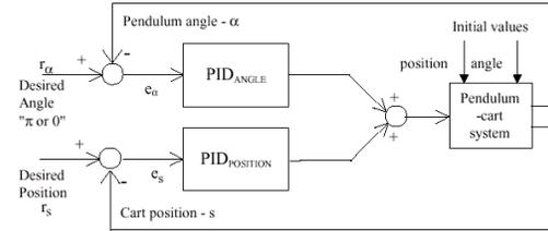
Fig. 13. Multivariable control system
