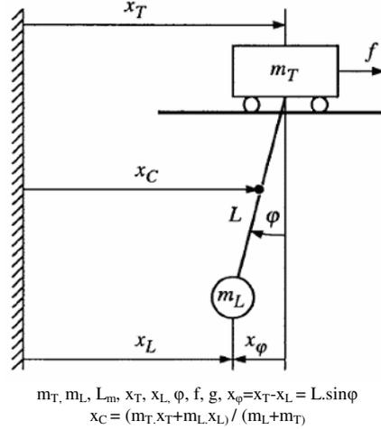
Fig. 10. Modeling crane trolley
