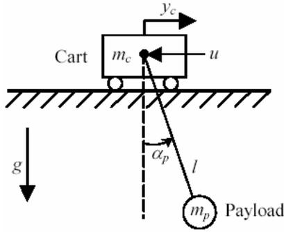
Fig. 3. Model of a gantry crane
