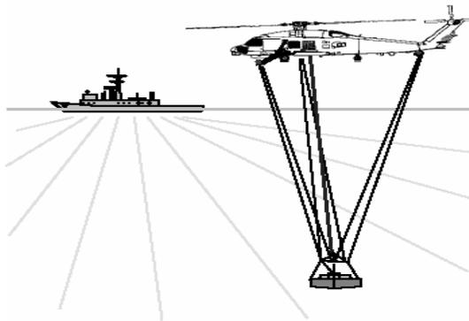
Fig. 20. Helicopter load transfer anti sway control
