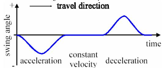
Fig. 15. Anti sway control and swing angle
