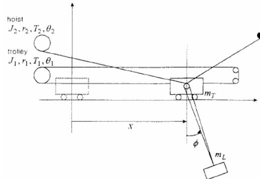
Fig. 2. Multiple rope anti-sway mechanism
