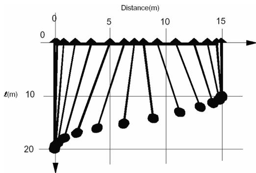
Fig. 6. Minimum time load transfer, smooth hoisting
